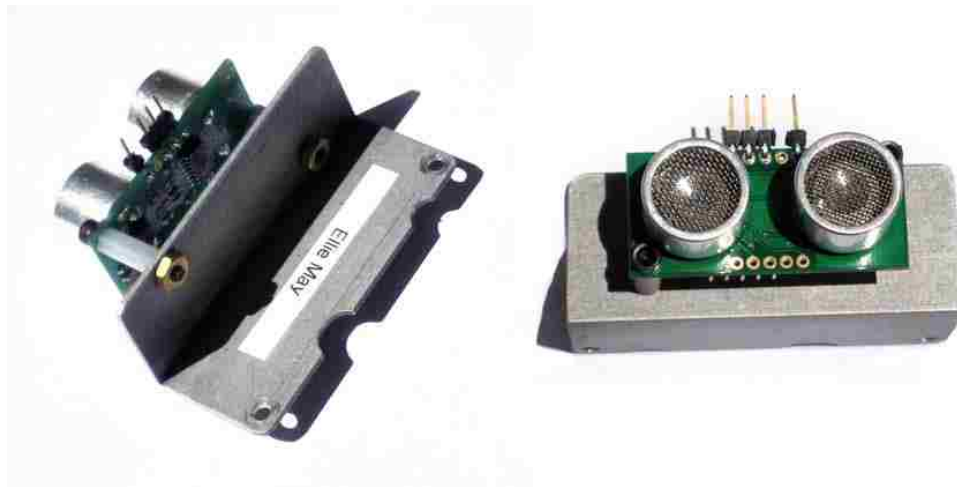
Figure 7 - SRF05 Ultrasonic with mounting bracket. Notches in bracket, near mounting holes, are relief for power switch and charging port.
