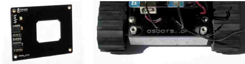
Figure 8 - RFID Module and rear of chassis showing mounting standoffs. Header pins, as supplied were right angle and changed to straight.
